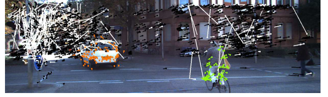
Fig. 3: Sparse optical flow vectors grouped by motion. Static points are shown in black, while the dynamic points are coloured by their cluster assignment. Points with low density in motion space (considered noise) are marked in white.
