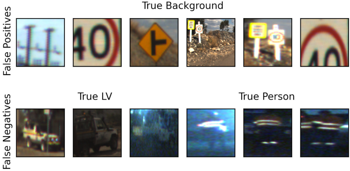
Figure 12: Validation samples where the nearest k-means background cluster model failed. Images are shown in their warped form, representing the DCN input. The four right false negatives were collected at night.
